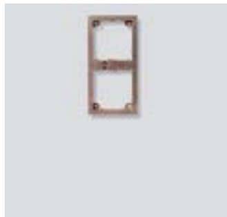
MR 611-2/1-0 Mounting frame made of zinc die-cast, to accommodate 2 function modules. Suitable for vertical or horizontal mounting. With quick-release screws for flush-mount housing and Siedle Vario key. Dimensions (mm) W x H x D: 99.5 x 199.5 x 17
