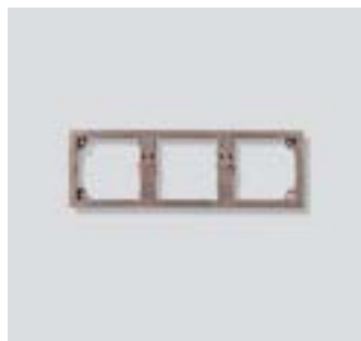
MR 611-3/1-0 Mounting frame made of zinc die-cast, to accommodate 3 function modules. Suitable for vertical or horizontal mounting. With quick-release screws for flush-mount housing and Siedle Vario key. Dimensions (mm) W x H x D: 99.5 x 299.5 x 17
