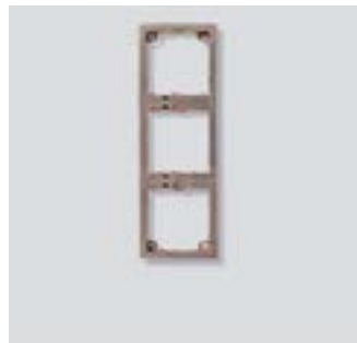
MR 611-3/1-0 Mounting frame made of zinc die-cast, to accommodate 3 function modules. Suitable for vertical or horizontal mounting. With quick-release screws for flush-mount housing and Siedle Vario key. Dimensions (mm) W x H x D: 99.5 x 299.5 x 17
