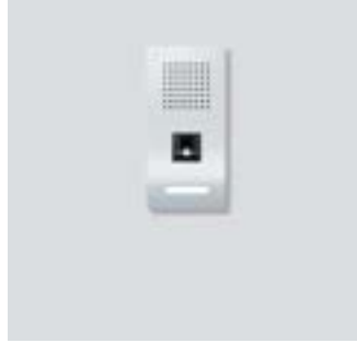
In-Home bus F CL AFPM 01 B-0 plug+play Classic door station for the In-Home bus with stainless steel front, brushed V4A. Door loudspeaker, 1 call button with backlit nameplate, exchangeable from the front. A fingerprint reader is also integrated as an access control system with LED. Ambient temperature: -20 °C to +55 °C
