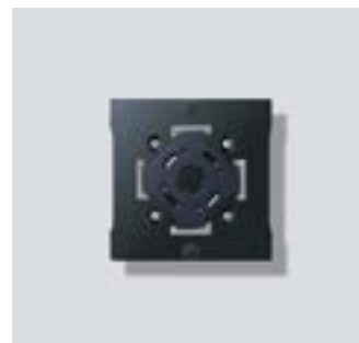
MA/LEDF 600-0 Mounting adapter LED surface area light to hold terminal blocks when an LEDF 600-... is mounted in housing BGA 611-..., BG/KSF 611-..., BG/SR 611-... or in the info sign housing of a KSF 61x. Fixture using the supplied adhesive tape. Dimensions (mm) W x H x D: 56 x 56 x 5.5
