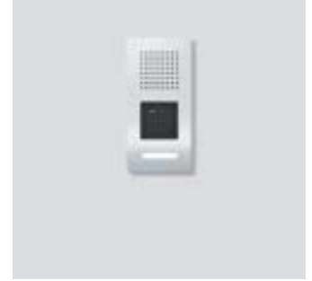
In-Home bus F CL AELM 01 B-01 plug+play Classic door station for the In-Home bus with stainless steel front, brushed V4A. Door loudspeaker, 1 call button with backlit nameplate, exchangeable from the front. An electronic key reader is also integrated as a no-contact access control system with function LED. The technical specifications of the electronic key reader correspond to the Vario ELM 600-... module. Ambient temperature: -20 °C to +55 °C
