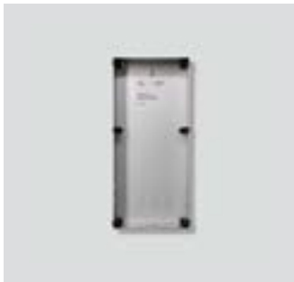
GU CL 06-0 Housing for flush-mounting made of hot-dip galvanised sheet steel. Matching housing must be ordered for each front panel. You can find the associated housing in the table. Dimensions (mm) W x H x D: 154 x 336 x 65
