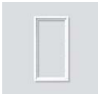
KR 611-4/2-0 Combination frames made of extruded aluminium sheath, powder-coated/painted, to surround the function modules and cover the plaster groove. A surrounding seal prevents the penetration of water. Dimensions (mm) W x H x D: 231 x 431 x 15
