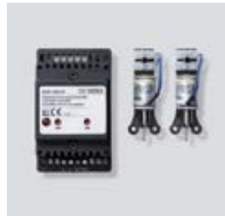
ZDS/CL Anti-pilfer accessory for mounting in the Siedle Classic door station as a concealed electromagnetic locking mechanism to secure the mounting screws. With anti-pilfer controller SDSC 602-01 in switch panel housing, for actuation of the anti-pilfer accessory ZDS/CL (for 1 pair), with status LED. Operating voltage: 12 V AC Operating current: max. 850 mA Protection system: IP 20 Ambient temperature: SDSC 602-01 0 °C to +40 °C, Locking -20 °C to +55 °C Horizontal pitch (HP): 3 Dimensions (mm) W x H x D: SDSC 602-01 53.5 x 89 x 60, Locking 25 x 70 x 32
